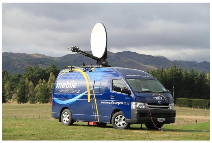
The van is equipped with iNetVu 1200 Satellite dish with iNetVu 7000 controller, and can operate from mains power, generator or onboard battery power. The van is also equipped as a mobile studio enabling MSS to have guest presenters conference to the rest of the network.
