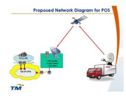
The mobile unit with C-COM's **iNetVu®** antenna system installed can be moved to any location in Malaysia. Once the vehicle reaches the site, a simple press of a button gets the antenna automatically pointed to the desired satellite. Traffic from the mobile unit goes up to the satellite and from there down to the Satellite HUB. From the HUB via a backhaul the traffic gets routed to their HQ.
