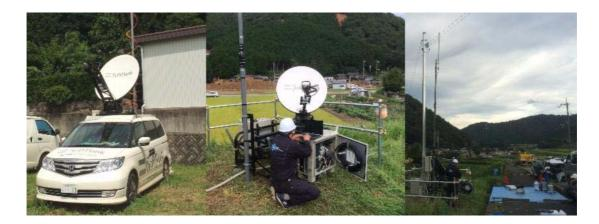
The transportable base station is equipped with the **iNetVu® 980 mobile antennas**. It is stocked in a warehouse before deployment, thus saving a number of vehicles from being occupied by the base station. Whenever it is needed, the antenna can be deployed quickly wherever it is required.
